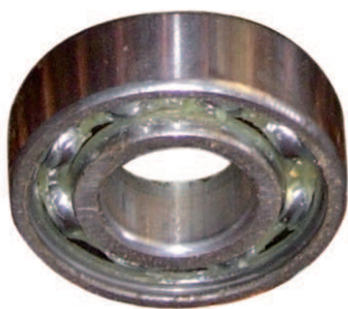
Fig. 9.16 : Ball bearings reduce friction
